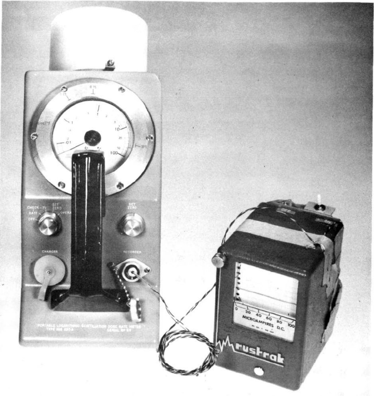
FIGURE 18. NIS 295 RADIATION SURVEY METER WITH "RUSTRAK" RECORDER
