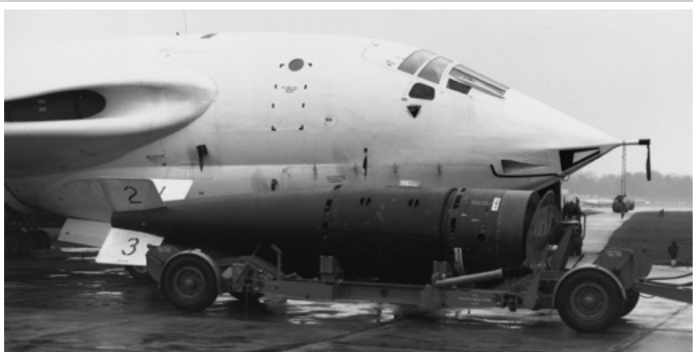
1960s A dummy Yellow Sun megaton free-fall bomb being tested with an RAF Victor bomber. RAF Bomber Command maintained Britain's strategic nuclear deterrent using weapons designed and developed by AWRE and assembled at the Royal Ordnance Factory at Burghfield until 1969
